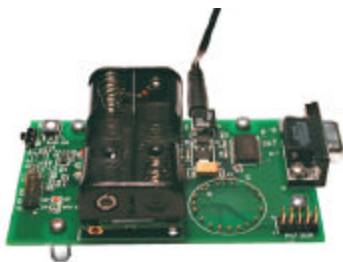
Fig. 2-2. MICA/MICA2 plugged into top-side of an MIB510
