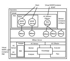
Fig. 1. Internal structure of the WSRF container
