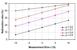
Figure 12: Impact of measurement errors on requestredirection ratio at different primary CDN load
