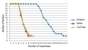
Fig 13. Number of machines varying during supesteps while running connected component algorithms on different datasets on iGiraph
