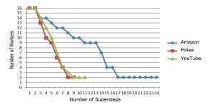
Fig 8. Number of machines varying during supesteps while running connected component algorithms on different datasets on iGiraph
