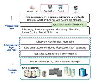
Fig. 1. Layerd design of Peer-to-Peer Grid architecture.
