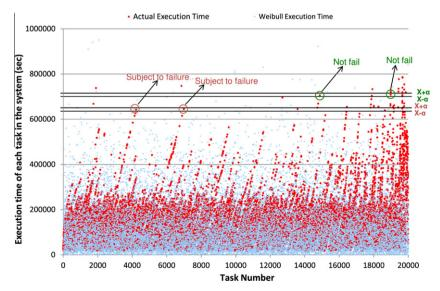
Fig. 3. Determination of tasks likely-to-fail based on the distribution of experimental and Weibull task execution time.
