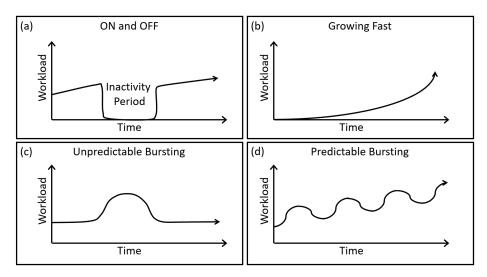
Fig. 3. Rough sketches presenting four workload patterns in cloud computing (a) ON and OFF, (b) Growing Fast, (c) Unpredictable Bursting, and (d) Predictable Bursting.
