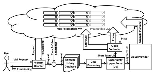
Fig. 4. A rough diagram representing the information flow in cloud management. The cloud controller requires one or more short-term uncertainty bounds for proper control. Long-term uncertainty bounds are useful in capacity planning for the future.
