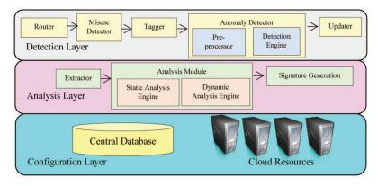
Figure 10. Layered architecture for detection of a zero day attack.
