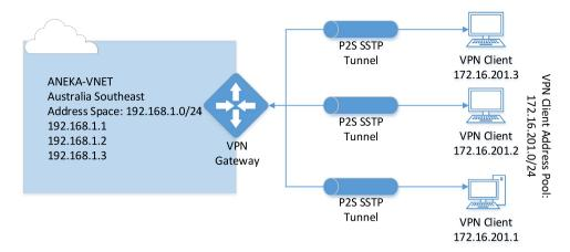
Fig. 4. A sample Azure Point-to-Site virtual network.
