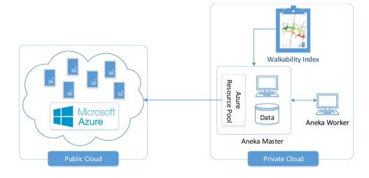
Fig. 5. Hybrid cloud testbed.
