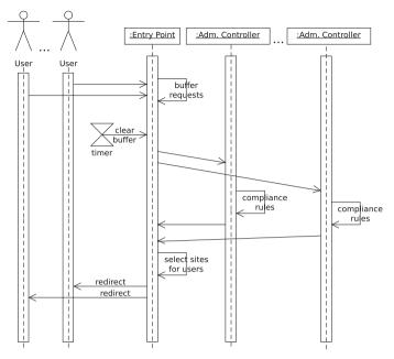
Fig. 3 Entry Point-Admission Controller interaction
