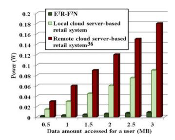
**FIGURE 5** Smart phone's power consumption in the proposed energy-efficient retailing using a femtolet-based fog network ( $E^2R$ - $F^2N$ ) and existing cloud server-based retail systems [Colour figure can be viewed at wileyonlinelibrary.com]
