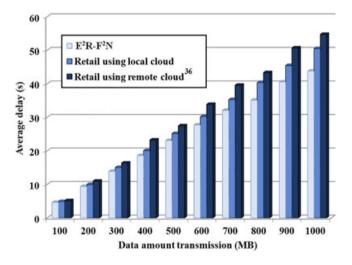
**FIGURE 9** Average delay in energy-efficient retailing using a femtolet-based fog network ( $E^2R$ - $F^2N$ ) and local cloud-based and remote cloud-based retail systems [Colour figure can be viewed at wileyonlinelibrary.com]
