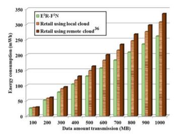
**FIGURE 11** Energy consumption in energy-efficient retailing using a femtolet-based fog network (E<sup>2</sup>R-F<sup>2</sup>N) and the local cloud-based and remote cloud-based retail systems [Colour figure can be viewed at wileyonlinelibrary.com]
