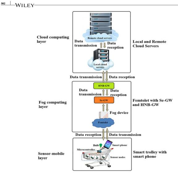
**FIGURE 1** Three-layer architecture of energy-efficient retailing using a femtolet-based fog network. HNB-GW, home node base station–gateway; Se-GW, security-gateway [Colour figure can be viewed at wileyonlinelibrary.com]
