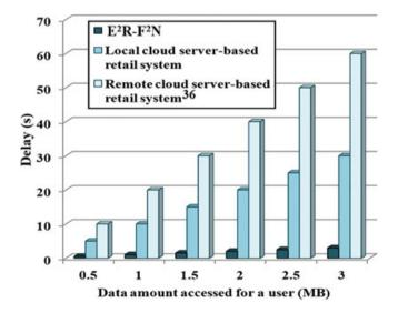
**FIGURE 4** Delay for a user in the proposed energy-efficient retailing using a femtolet-based fog network ( $E^2R$ - $F^2N$ ) and existing cloud server-based retail systems [Colour figure can be viewed at wileyonlinelibrary.com]
