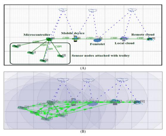
**FIGURE 6** A, Energy-efficient retailing using a femtolet-based fog network scenario created in QualNet 7; B, Simulation scenario during execution [Colour figure can be viewed at wileyonlinelibrary.com]
