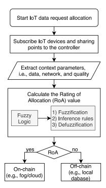
Fig. 3. Flowchart of the data allocation mechanism.
