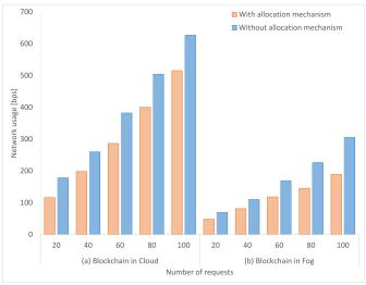
Fig. 11. Network usage in bits per second—with/without the allocation mechanism in (a) blockchain-based cloud and (b) blockchain-based fog.
