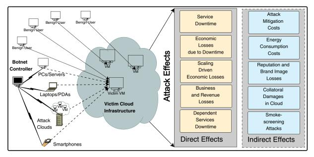
Fig. 2. DDoS attack in cloud: direct and indirect effects.
