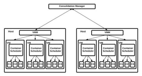
Figure 8. A common architecture for the studied use cases: VMM sends the data including the status of the host along with the list of the containers to migrate to the consolidation manager. The consolidation manager decides about the destination of containers and sends requests to provision resources to the selected destination.
