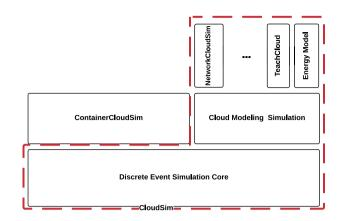
Figure 3. ContainerCloudSim relations to the CloudSim ecosystem. [Colour figure can be viewed at wileyonlinelibrary.com]
