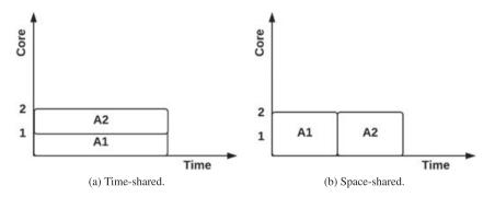
Figure 6. Time-shared and space-shared provisioning concepts for containers A1 and A2 running on a VM.
