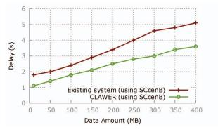
Figure 5: Delay in proposed CLAWER framework (indoor)
