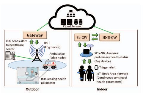
Figure 2: CLAWER: Hierarchical Placements of IoT/ Edge/ Fog/ Cloud
