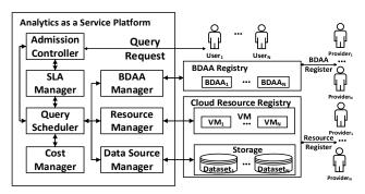
Figure 1. Architecture of the AaaS Platform
